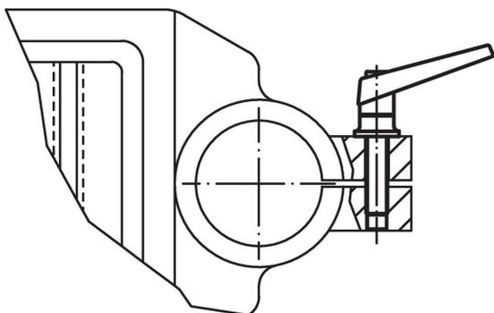
Increase of clamping force with axial bearing
