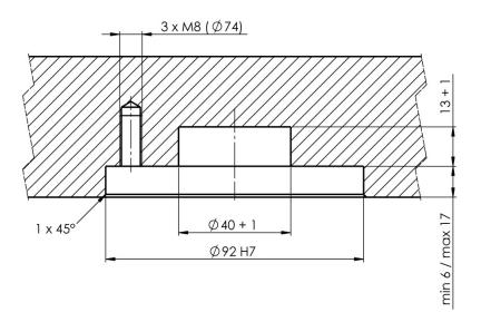
Mounting depth Connecting Element and Connecting Ring:
