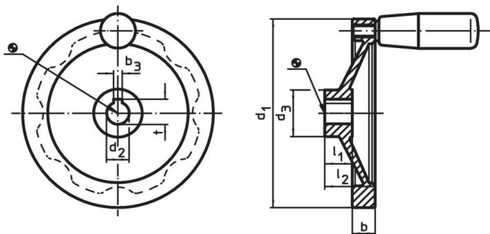
The orientation of the hub keyway may be different than shown in the drawing.
