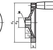
The orientation of the hub keyway may be different than shown in the drawing.
