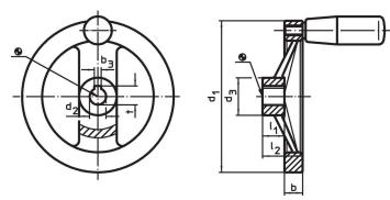
The orientation of the hub keyway may be different than shown in the drawing.
