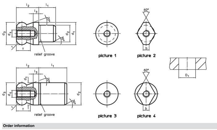
Location hole Dimensions Art. No. P - $D_1$ d<sub>3</sub> d₁  $d_2$  $d_4$ l<sub>2</sub> I<sub>1</sub> I<sub>3</sub> t r H7 g6 n6 -0.01 -0.05 [mm] [mm] [g] with ball end plain - picture 1, Tool steel 22630.0320 20 14 20 M5 14 20 5 10 5 14 58
