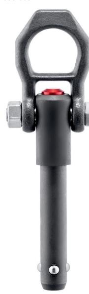
Heavy-duty lifting element for quick and easy use, with moveable shackle and locking stud to provide protection against unintentional unlocking. Special lifting devices, e.g. threads for ring bolts, are no longer required on the workpiece.
