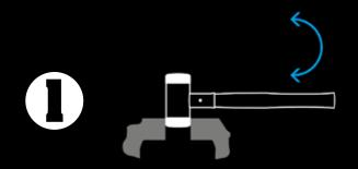
Firmly clamp the used insert in a vice and loosen with a lateral twisting movement.
