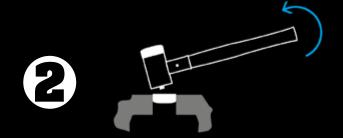
When the insert is loosened, pull the mallet upwards.
