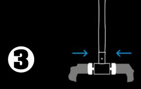
In the vice, press the new insert into the housing and insert retaining pins.
