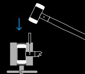
**1** Clamp the hammer securely into a vice and tap out the clamping pin using a pin punch.
