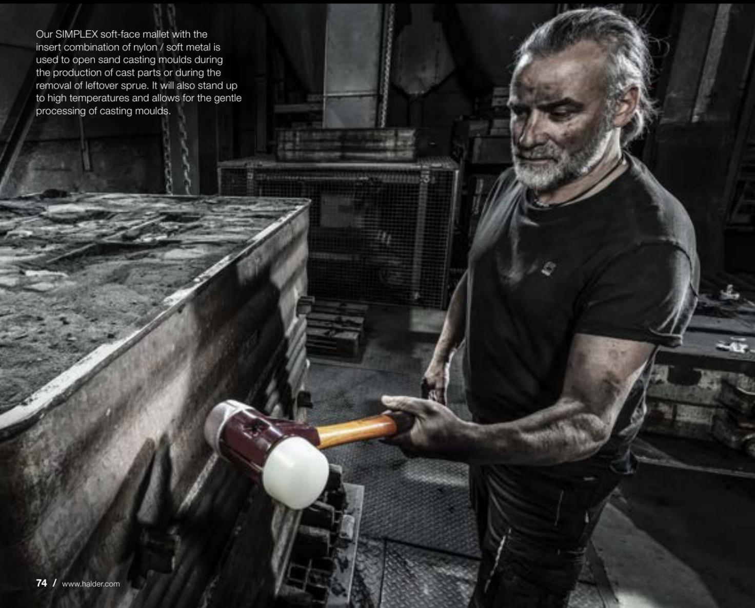
Our SIMPLEX soft-face mallet with the insert combination of nylon / soft metal is used to open sand casting moulds during the production of cast parts or during the removal of leftover sprue. It will also stand up to high temperatures and allows for the gentle processing of casting moulds.
