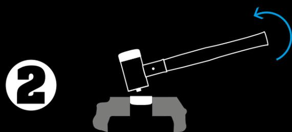
**2** When the insert is loosened, pull the mallet upwards.
