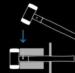
**6** Tap the clamping pin into the bore hole.
