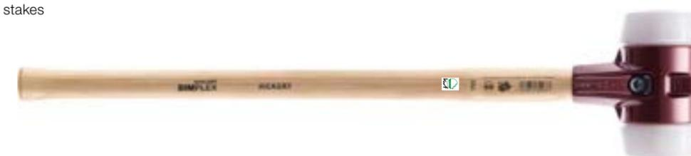
Wooden stakes will splinter if driven in with steel hammers or soft-face mallets whose head diameter is too small. This is why HALDER offers the SIMPLEX sledge hammer with superplastic inserts and an extra large diameter of 125 mm. The non-rebound forestry sledges deliver increased impact force, while their completely flat nylon inserts prevent the stakes from splintering.
