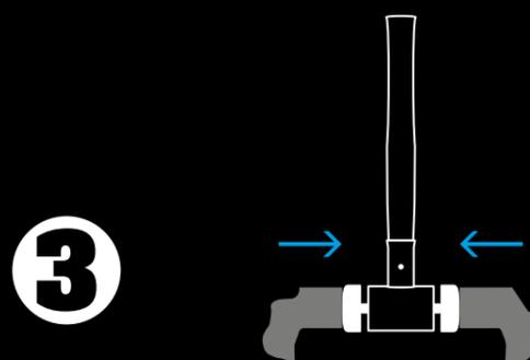
**3** In the vice, press the new insert into the housing and insert retaining pins.
