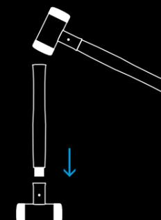
**4** Clamp the hammer securely into a vice and tap the handle into the body using the aluminium wedge.
