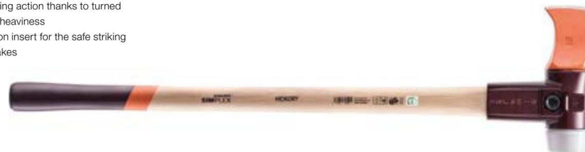
The SIMPLEX splitting maul is the tool of choice for log splitting. The drop-forged splitting insert delivers extremely high splitting action thanks to its turned nose. This effect is amplified by its total weight of 4,100 g and high top heaviness. The protective insert on the opposite side makes it possible to wedge wood open in a safe and gentle manner and without the need to rely on a second tool!
