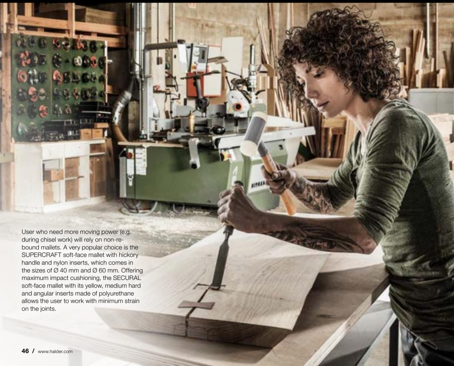
User who need more moving power (e.g. during chisel work) will rely on non-rebound mallets. A very popular choice is the SUPERCRAFT soft-face mallet with hickory handle and nylon inserts, which comes in the sizes of ∅ 40 mm and ∅ 60 mm. Offering maximum impact cushioning, the SECURAL soft-face mallet with its yellow, medium hard and angular inserts made of polyurethane allows the user to work with minimum strain on the joints.
