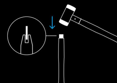
**3** Tap an aluminium wedge into the slot found in the wooden handle.
