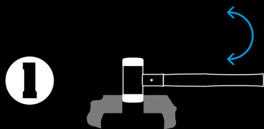
**1** Firmly clamp the used insert in a vice and loosen with a lateral twisting movement.
